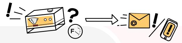
If the generator fails to start due to a malfunction, no fuel or for any other reason preventing startup, the V2 controller will enter an Error State and send a notification via email to inform of the startup error. Controller must be reset(via app) or power cycled after inspection to continue Auto Start/Stop Mode.
