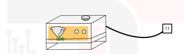
Connector **11** must be connected to Generators 12vdc output or to charging wire for generators starter battery. If you are receiving a +12v signal while engine is **NOT** running on this connector, a blocking diode must be placed between charging wire and starter battery positive terminal.
