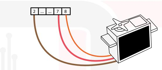
Choke Servo Connectors are 2, 7, 8 on V2 AutoGen
