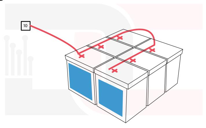
Connector **10** must be connected directly to the positive terminal of battery bank. Best practise is to connect directly on positive battery terminal to avoid any voltage drop.
