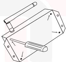
1. Remove the 4 screws of rear panel. Carefully open box not to dislodge the external wifi antenna cable.
