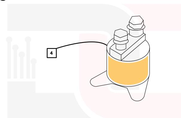
Connector **4** must be connected to generators starter motor solenoid relay. This sends a +12vdc signal to starter relay. Bypass or Tap into Start Switch or Key Switch on generator and connect starter motor relay signal wire directly to connector **4**.
