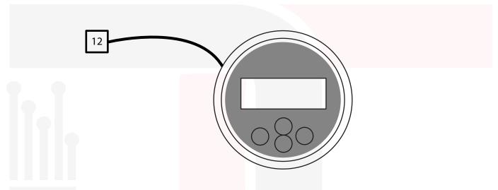
Connector **12** must be connected for example: to BMV-700 relay output or from majority of chargers/inverters with programmable AUX output to signal Charged Battery Status.
