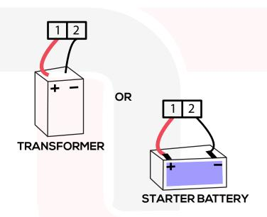
Connections  ${\bf l}$  and  ${\bf 2}$  are for powering the controller from a 12v dc source. You can use the 12v starter battery as the power source or an external 12v - 2000mA transformer. A small 12v trickle charger connected to mains for keeping starter battery full is best practise. Connector  ${\bf l}$  is +12v and Connector  ${\bf 2}$  is -12v (ground also to generator)
