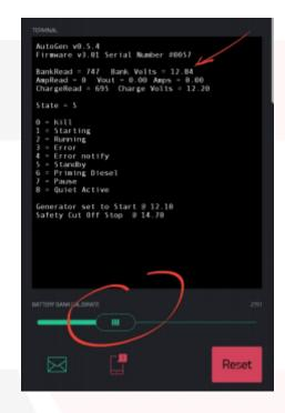
First step within the app is to scroll down to the bottom of the apps screen and adjust the battery bank calibrate slider as pictured below. Match the controllers Bank Volts with your other measuring equipment, multimeter etc.
