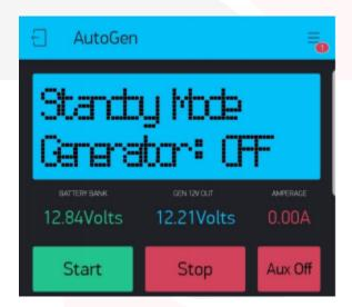
**Note**: If you notice a Red indicator on top right hand screen of app, review step 3 as this means that the controller is unable to access the internet.
