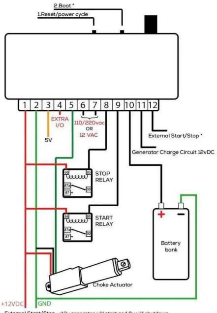
External Start/Stop: +12v generator will start and 0v will shutdown 2.Boot: (hold 3 seconds for OTA update or 10 seconds for clear stored wifi credentials)
