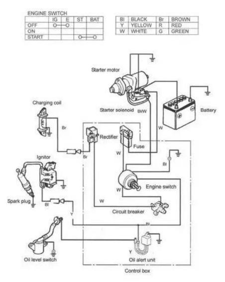
Here we can see that the engine switch contacts IG and E are closed to shut down the engine and ST and BAT are closed to start the engine.
