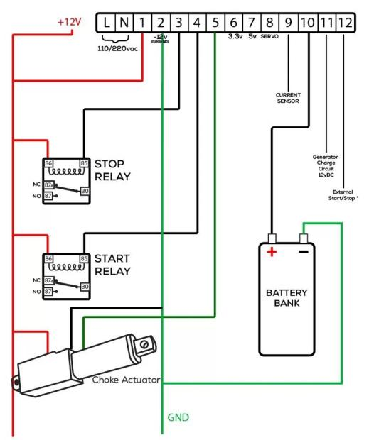
The actuator is prewired with a DPDT(double pole double throw) relay. Red wire is connected to constant +12vdc, Black wire is connected to GND and the Green wire is connected to pin#5.
